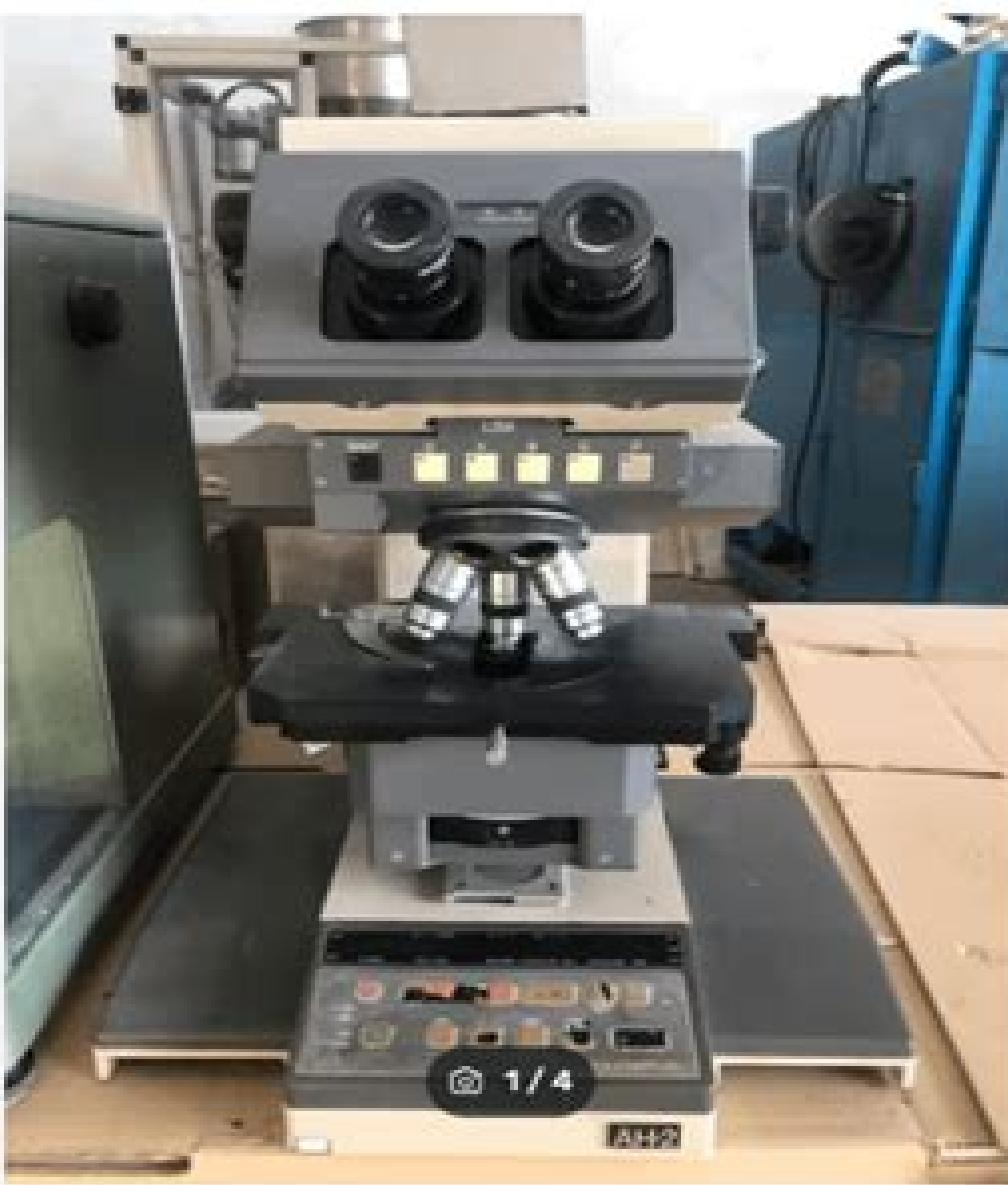
MICROSCOPIO OLYMPUS VANOX-T AH2
