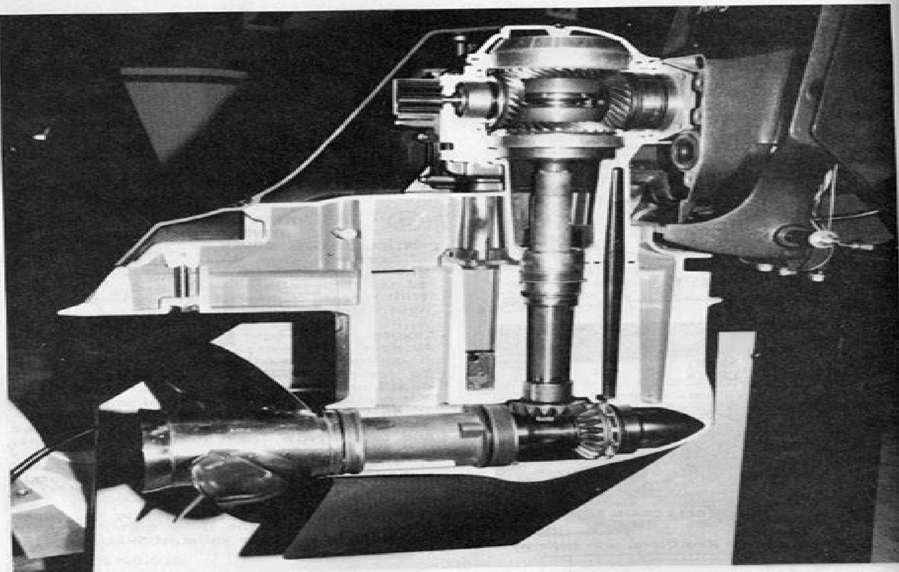
Manufacturer's cutaway unit exposing major parts of the upper gear housing, the drive shaft, and the lower unit, including the propeller. A view, such as this, is an excellent educational tool to understand and appreciate how the various components interact to move the boat. Once an individual has worked on internal parts of the stern drive — following the procedures presented in this manual — he/she should be able to accurately identify and describe almost all units or assemblies visible.
