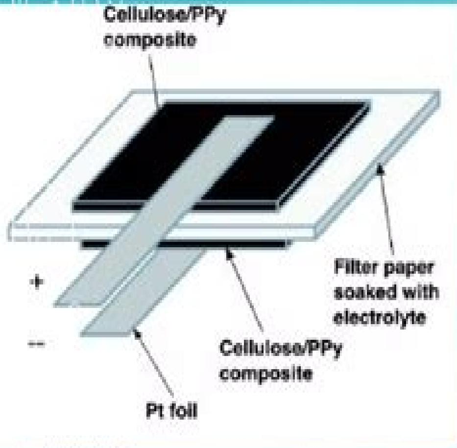
A paper battery construction involves the following components:
