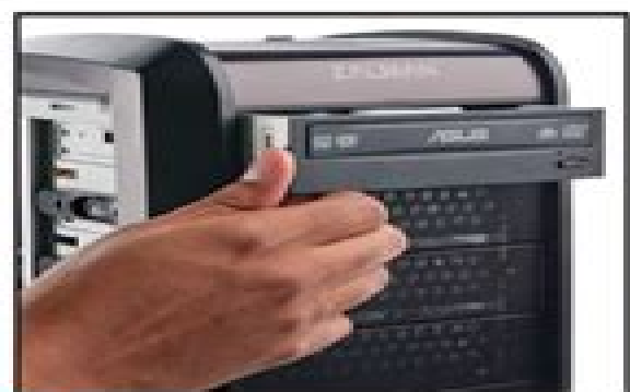
7 Install the optical drive
