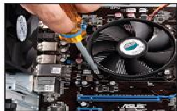
4 Mount the CPU cooler
