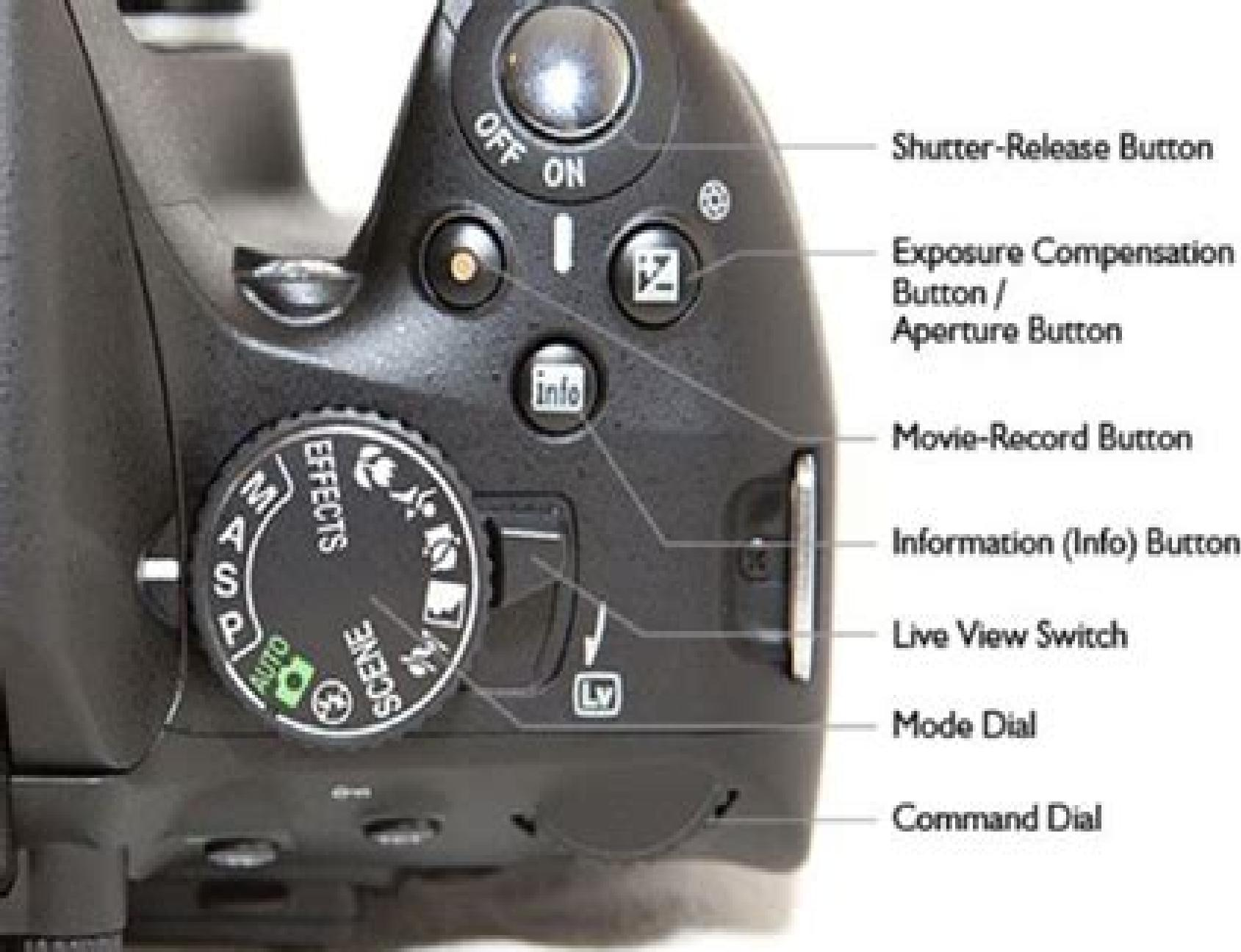
Figure 2 - Controls on the top of the D5100
