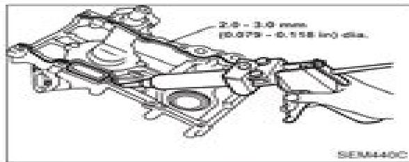
6. Apply a continuous bead of liquid gasket to front cover.
