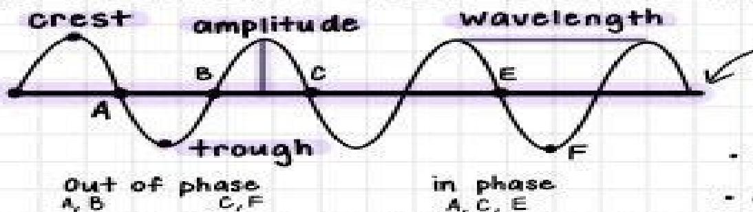
Frequency  $f$  describes the number of waves per second. measured in Hertz (Hz)
