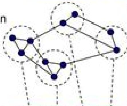
**Parallel simulation** involves the execution of a *single* simulation program on a collection of *tightly* coupled processors (e.g., a shared memory multiprocessor).
