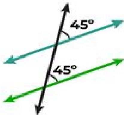
The given lines are parallel because a pair of corresponding angles are equal.
