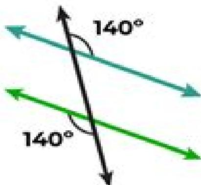
These lines are parallel because a pair of alternate interior angles are equal.
