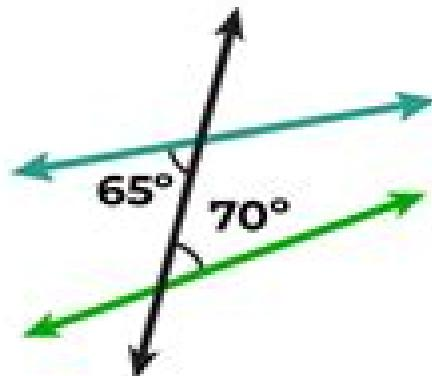
These lines are not parallel because the alternate interior angles are not equal.
