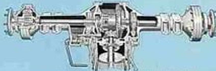
Ruggedly cast rear axle has final reduction through totally enclosed oil bath epicyclic hub gears giving road drive reduction of 1:19.5. Note also the two implement mounting pads and differential lock fast pedal. Disc brakes, acting independently, are sealed against weather, give double quick service.
