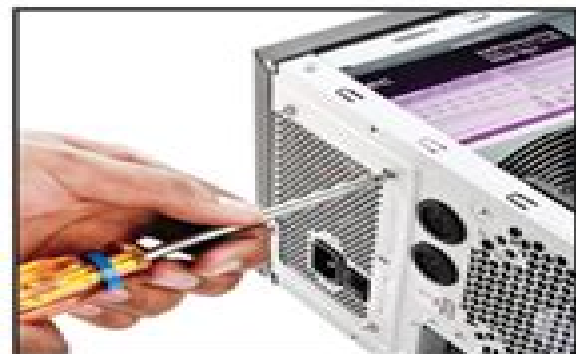
1 Install the power supply
