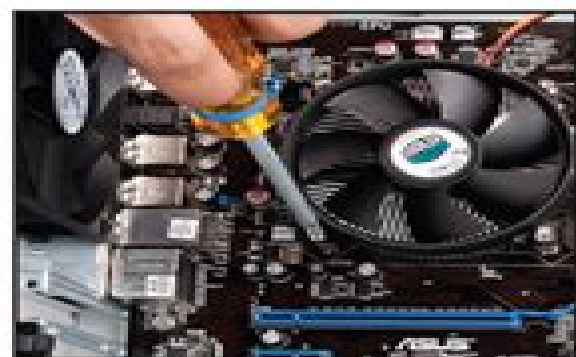
4 Mount the CPU cooler
