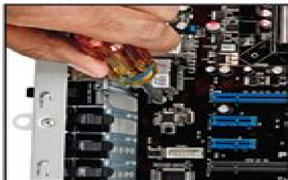
2 Install the motherboard
