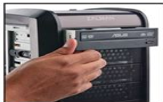
7 Install the optical drive
