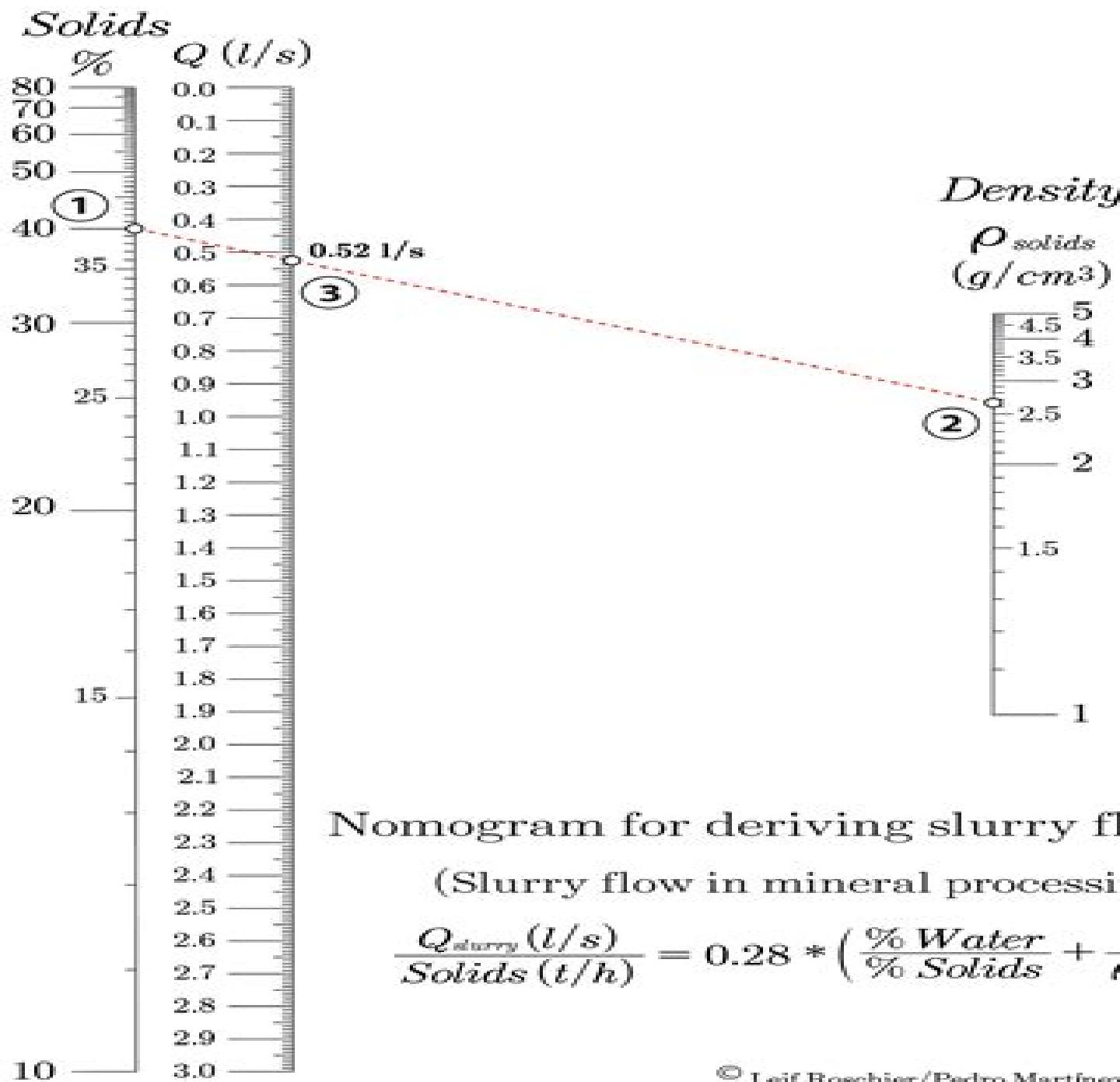
Nomogram for deriving slurry flow ( $Q$ )
