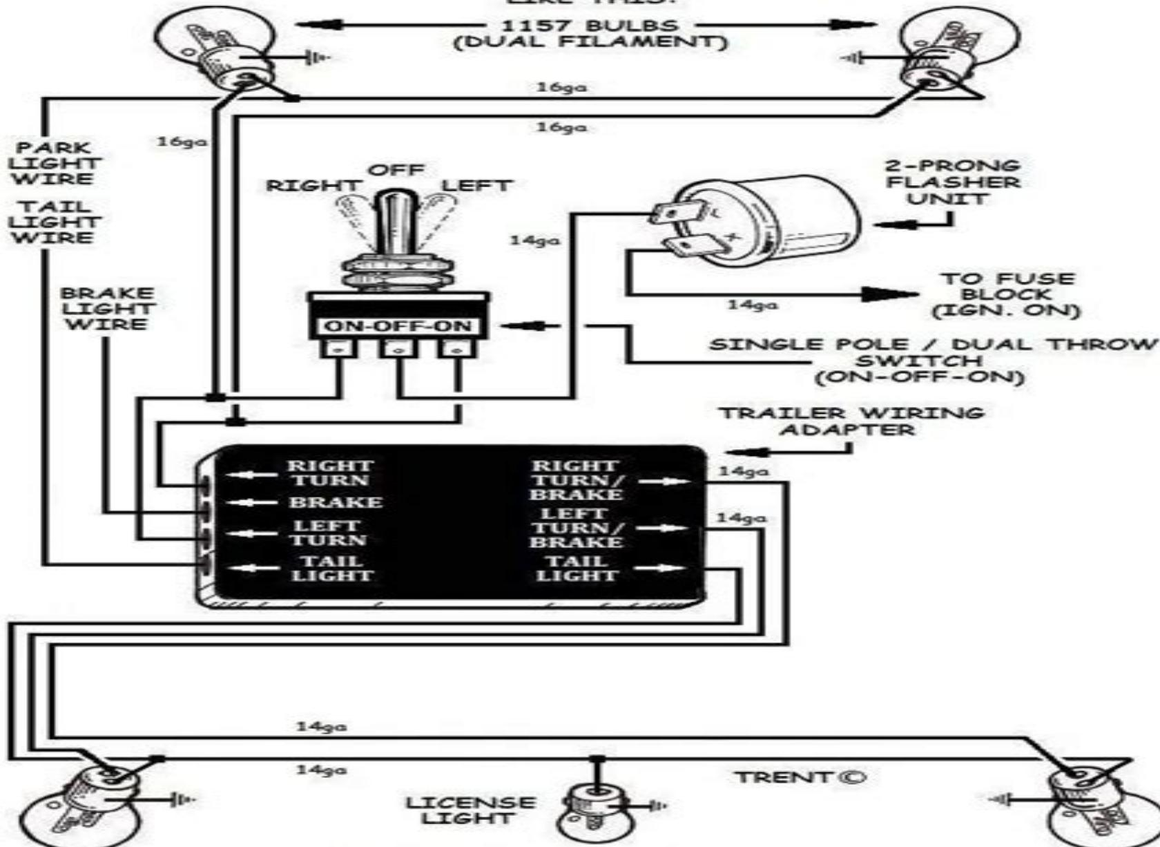
\* REAR BULBS (1157) HANDLE BRAKE, TURN, AND TAIL WIRED THIS WAY...
