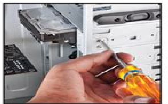
6 Install the hard drive
