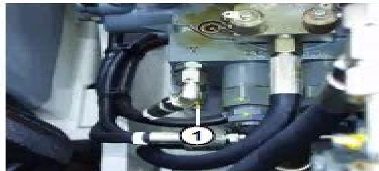
10. Set the pressure for TC-valve at the measuring union "slew to right" (M9) to the specified value by screwing in/out the screw (1), while the "slew to right" function is activated.
