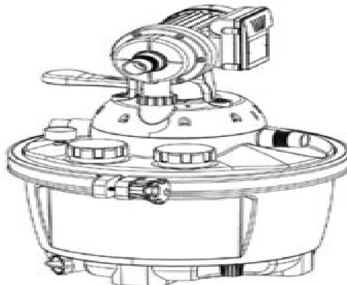
*Sand not included. USE ONLY No. 20 Silica Sand with a particle size of 0.45 mm – 0.55 mm*
