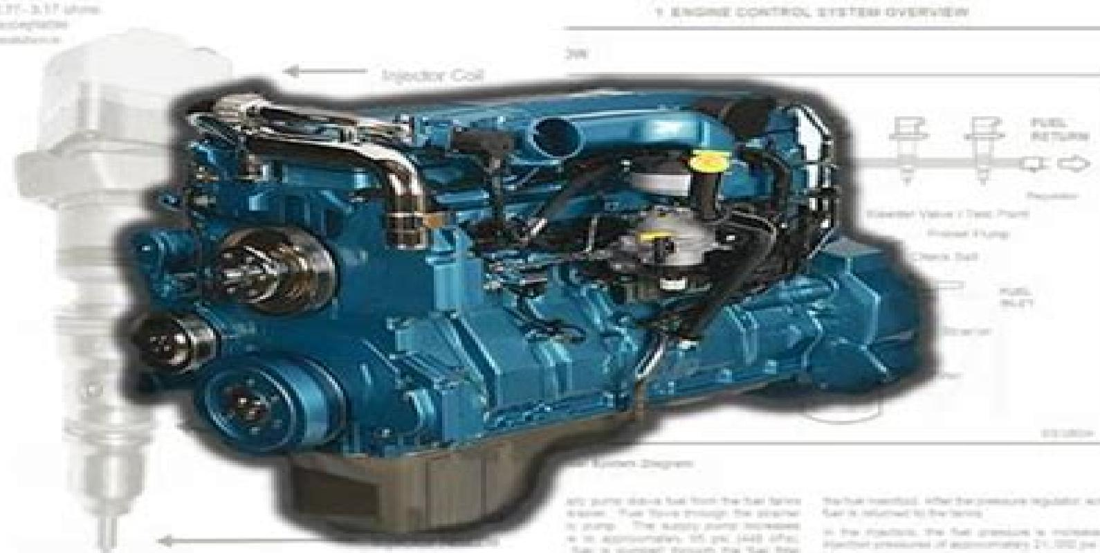
fuel pump draws fuel from the fuel filter system. Fuel flows through the pressure fuel pump. The output pump increases the pressure to approximately 105 psi (4450 kPa). Fuel is pumped through the fuel line assembly (not shown) for distribution through the lines to the fuel injectors.
