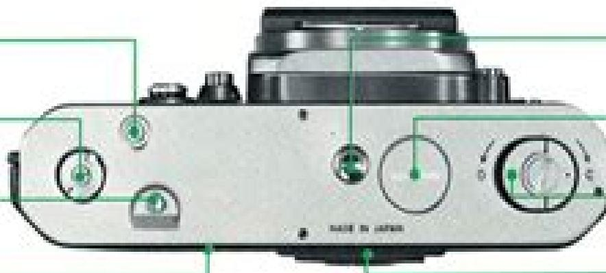
\*Film-advance coupling: connects with the drive shaft of the motor drive.
