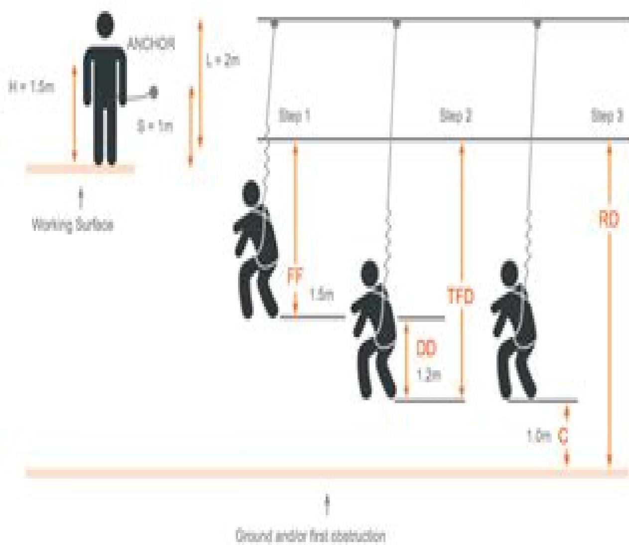
Free fall (FF) = lanyard length (L) + distance from anchor to platform (D) + height of lanyard attachment to harness (H).
