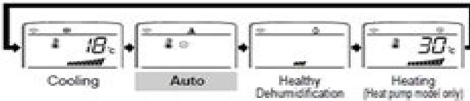
**3** The temperature and fan speed are automatically set by the electronic controls based on the actual room temperature. If you want to change the set temperature, close the door on the remote control and press the Room Temperature Setting buttons. The cooler or warmer you feel, the more times (up to two times) you should press the button. The set temperature will then be changed automatically.
