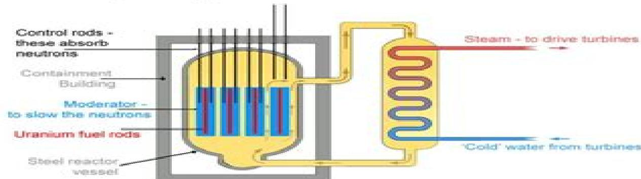
(i) Which part of the reactor is designed to control the rate of nuclear fission?
