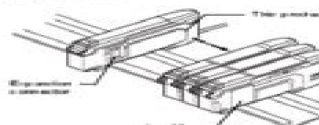
**Notes:** Do not pull this product out when connecting or disconnecting. If this product is pulled out while it is being connected or disconnected, this product will be damaged, causing the connection to fail.
