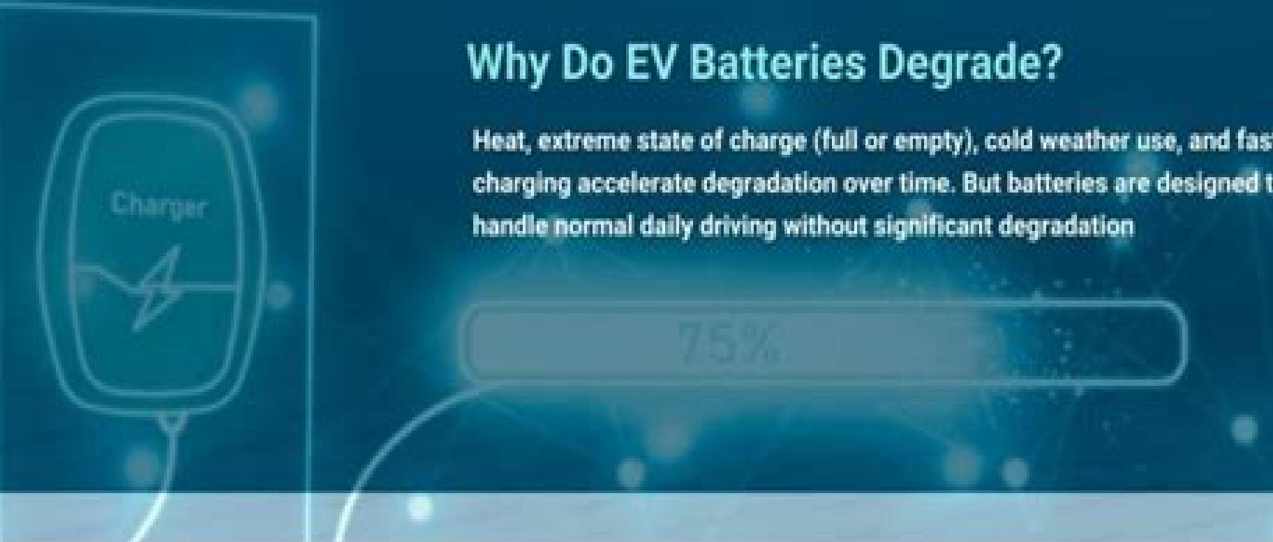
Heat, extreme state of charge (full or empty), cold weather use, and fast charging accelerate degradation over time. But batteries are designed to handle normal daily driving without significant degradation
