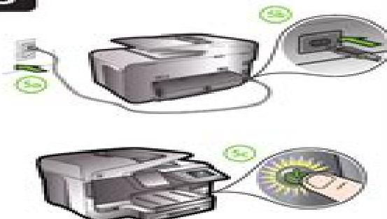
Connect the power cord and turn on the printer.
