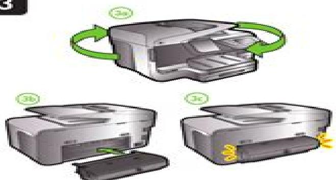
Install the HP automatic two-sided printing accessory (duplexer).
