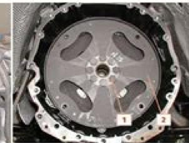
4. Undo all the fastening screws (1) and remove the complete engine flywheel (Flexplate) (2).
