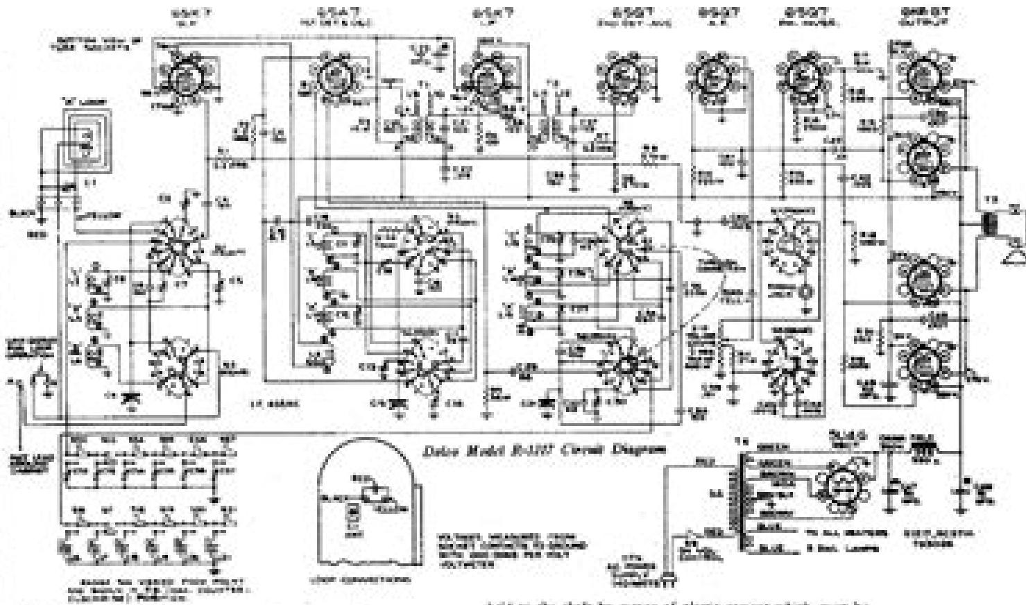
**Two-Quadrant.**—For all alignment operations, connect the low side of the non-oscillate to the receiver chassis, and keep the output as low as possible to avoid a-v-c action.
