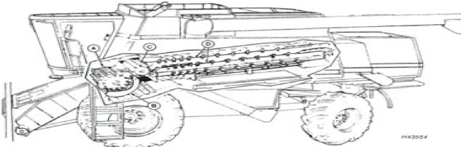
Cut crop is fed up the feeder house then through the cylinder (A) and concave (B).
