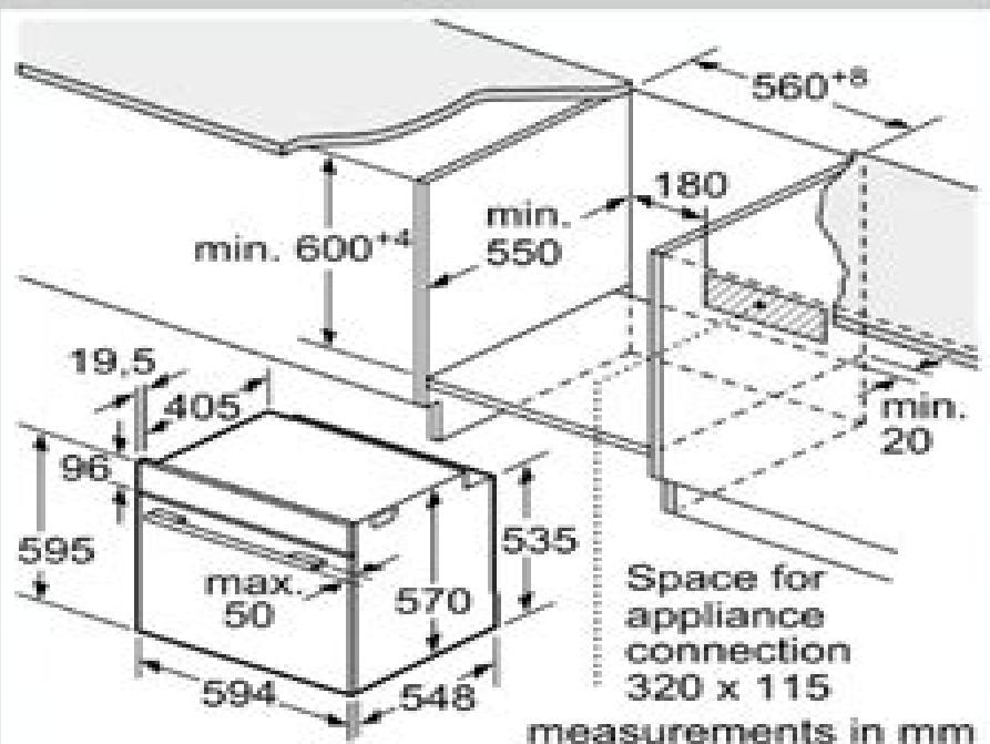
measurements in mm
