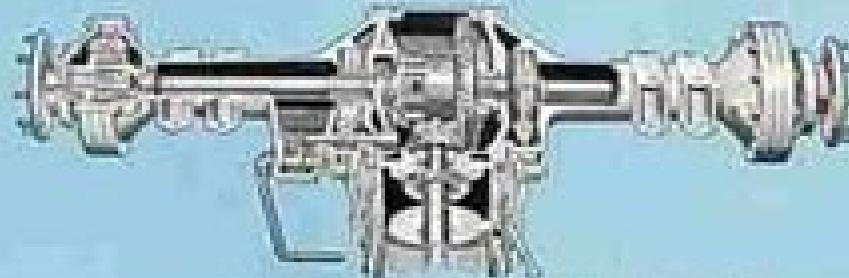
Ruggedly cased rear axle has final reduction through totally enclosed oil bath epicyclic hub gears giving road drive reduction of 1:19.5. Note also the two implement mounting pads and differential lock fast pedal. Disc brakes, acting independently, are sealed against weather, give double quick service.
