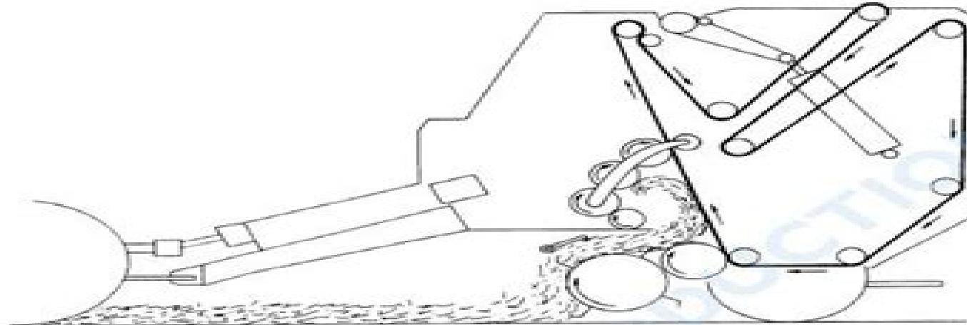
The **PICKUP** feeds material back to the floor roll. The **WINDGUARD** holds material for positive feeding. The **FLOOR ROLL** feeds material to the **BELTS**, which move material to the core-forming area. The **FORMING ROLLS** assist in curling the material and starting the core.
