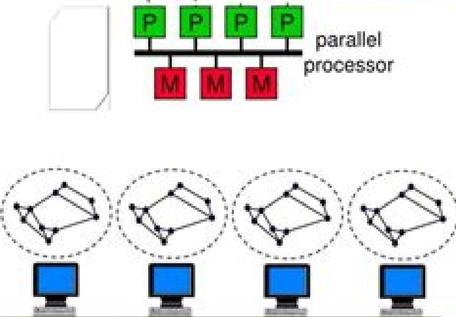
**Replicated trials** involves the execution of *several*, independent simulations concurrently on different processors
