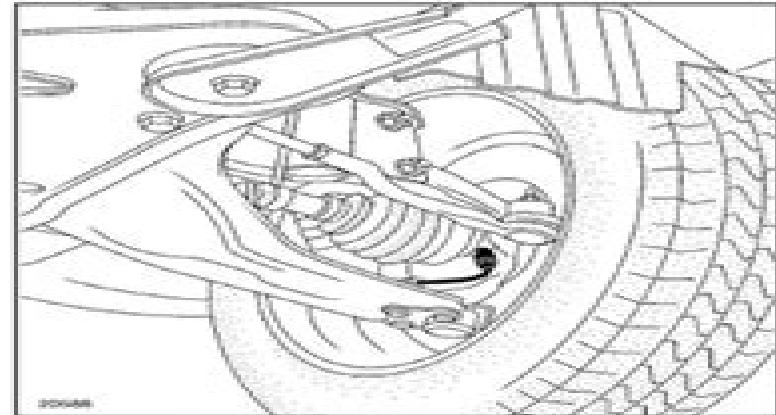
Unclip the wheel sensor ABS equipment.
