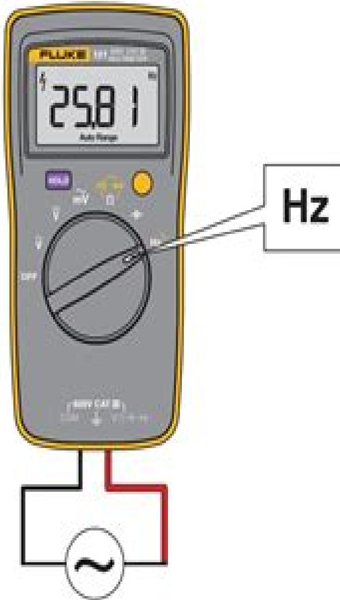
Figure 4. Measure Frequency/Duty Cycle
