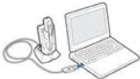
2 Connect USB connector to a free USB port on your computer. A USB hub can be used but ensure that it can supply sufficient power (500 mA) to charge the headset.
