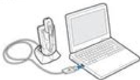
Connect USB connector to a free USB port on your computer. A USB hub can be used but ensure that it can supply sufficient power (500 mA) to charge the headset.
