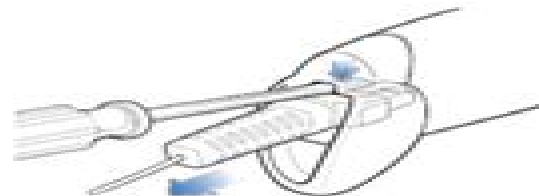
Remove Cable (to change interface)
