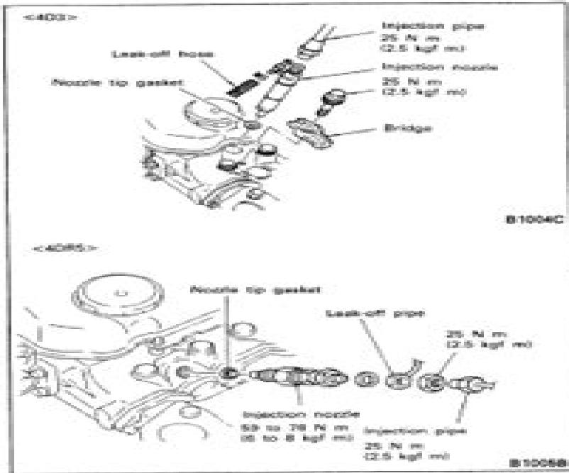
Check the injection start pressure and spray condition of the injection nozzle. If not as specified, perform the following operations.
