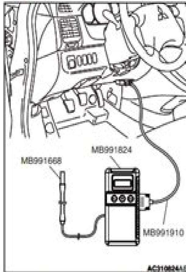
To prevent damage to special tool V.C.I. (MB991824), always turn the Ignition switch to the "LOCK" (OFF) position before connecting or disconnecting special tool V.C.I. (MB991824).
