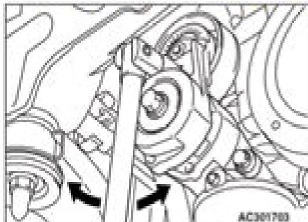
3. Securely insert the spindle handle or ratchet handle with a 12.7 mm insertion angle into the jig hole of the auto tensioner. Turn the auto-tensioner to the left and right to check and see that there is no threading.
