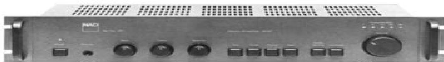
The NAD 3020 is a no-frills, moderately-priced amplifier designed to provide state-of-the-art performance at volume levels far in excess of what would be expected from its conservative 20-watt per channel power rating. This remarkable characteristic is made possible by high-voltage, high-current output stages which can deliver short-term bursts of two to five times the rated continuous power output into loudspeakers of widely varying impedances.
