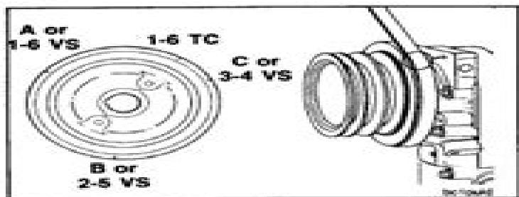
**Injector and Valve Adjustment Sequence**
