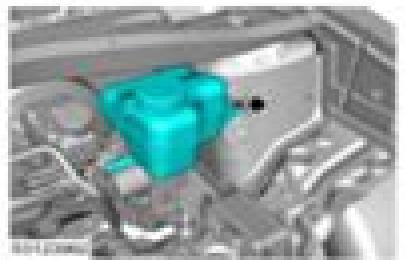
5. Loosen the clip and remove the coolant expansion tank.
