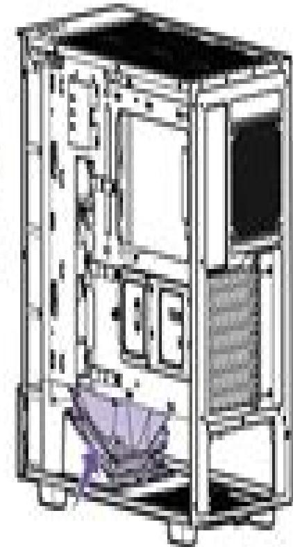
③ From the front side of the shroud, lift the air duct and release it from the case.
