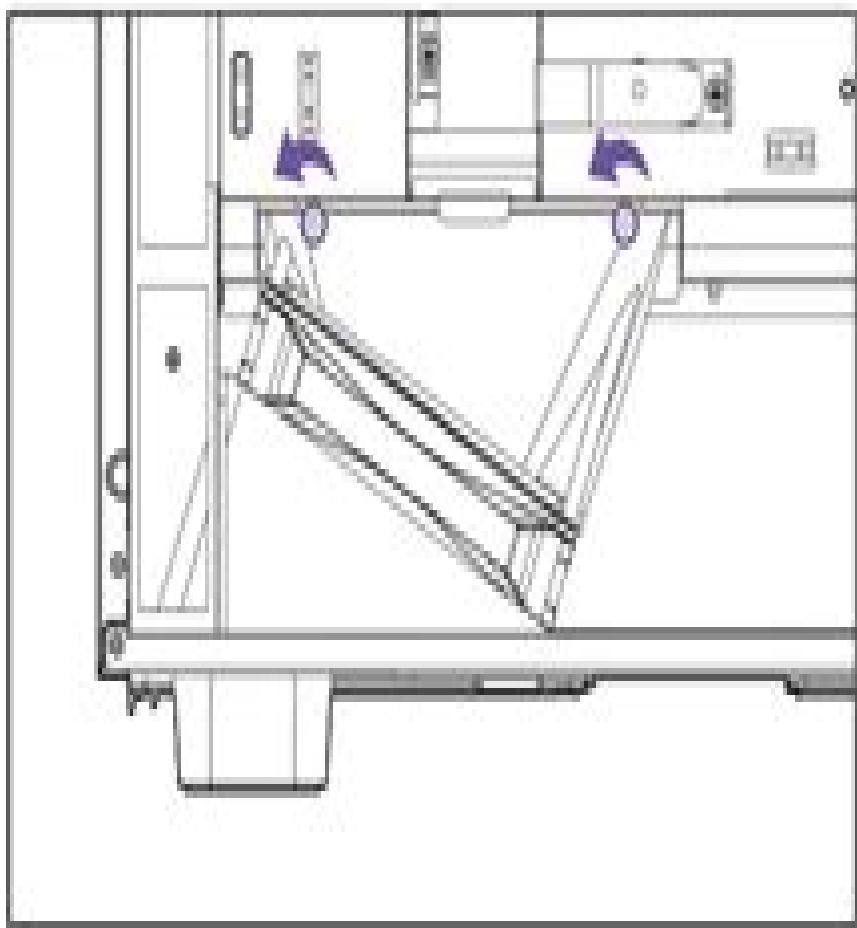
② From the rear side of the PSU shroud, push and lift on the air duct as indicated to release the air duct and bottom fan.
