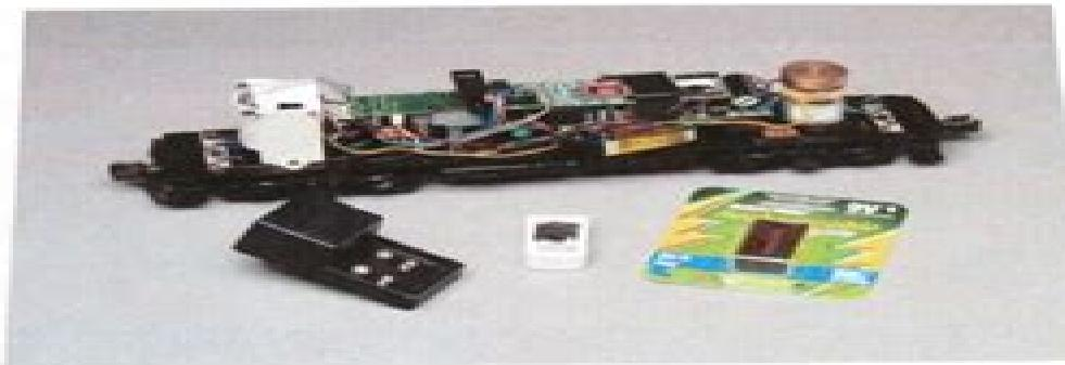
Although MTH circuitry continuously recharges the battery whenever you run your locomotive, the original factory-installed NiCad (nickel cadmium) battery deteriorates with age until it can no longer hold a charge or reach its full voltage capacity, no matter how long you charge it. At this point, the battery must be replaced.
