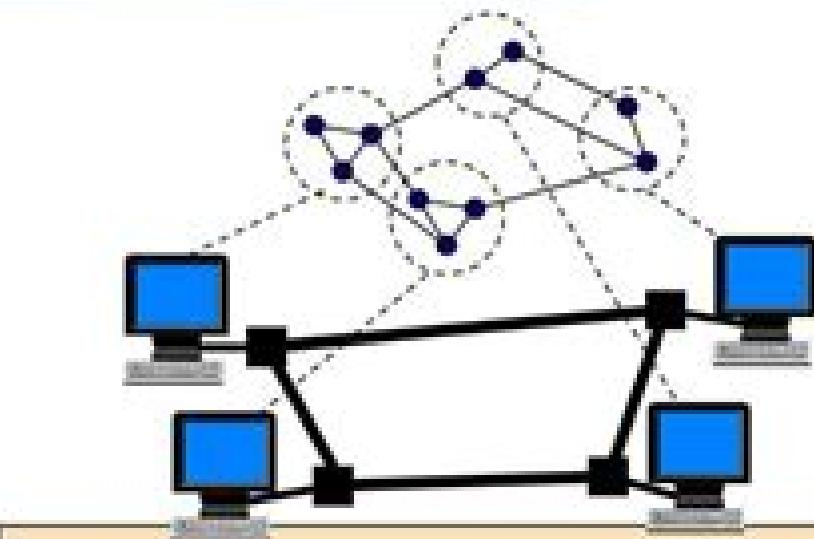
**Distributed simulation** involves the execution of a *single* simulation program on a collection of *loosely* coupled processors (e.g., PCs interconnected by a LAN or WAN).
