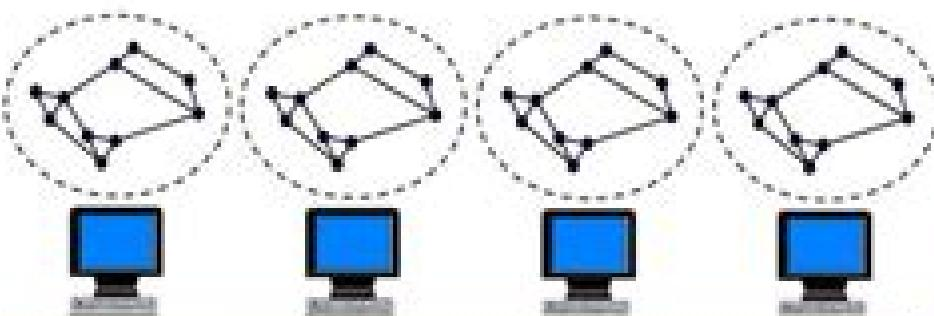
**Replicated trials** involves the execution of *several*, independent simulations concurrently on different processors
