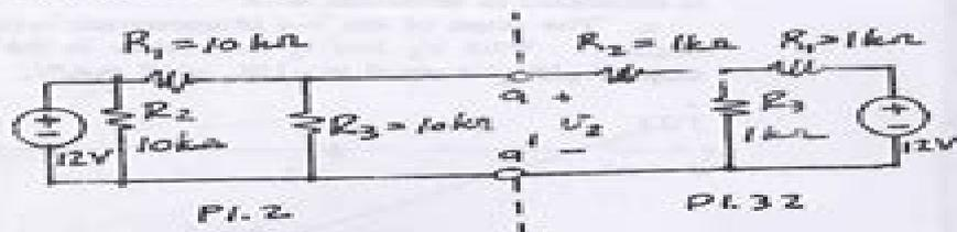
As a first step, the Thévenin equivalent of each half of the circuit is taken, as shown below.
