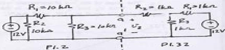
As a first step, the Thévenin equivalent of each half of the circuit is taken, as shown below.
